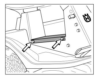
2. Check the tension of the steering wires by pushing them together as shown in the diagram. It should be possible to push them together so that the distance between them is half as much, without using unnecessary force.
